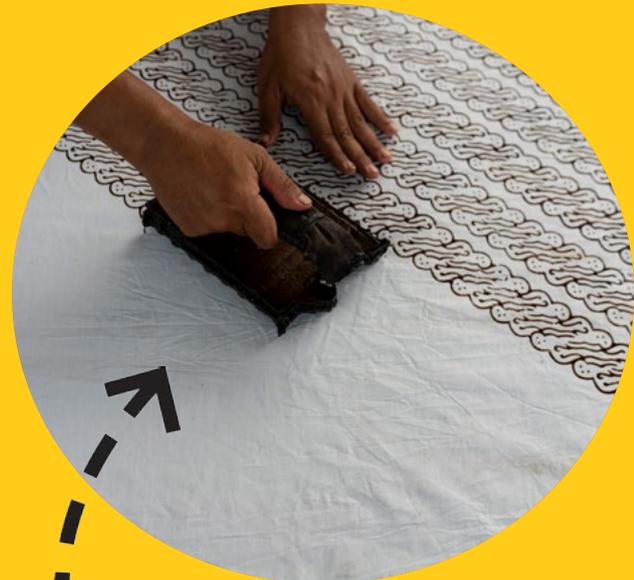
This wax resist and dyeing process is often repeated on the one piece of fabric, to create a more intricate design. A new layer of wax will preserve the fabric's colour before it is dyed again. After the final dyeing the fabric is boiled to remove the wax, revealing the completed textile.
